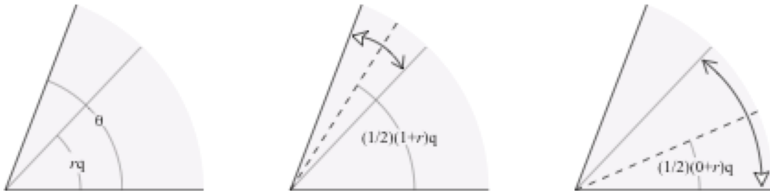
Figure 30. Division of an angle by bisection corresponds to the two operations that make up the binary folding method.
